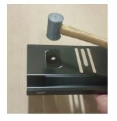
1.) Punch out washer from the mailbox plate. Only one is required for assembly. Use a small hammer to gently knock it out or push with your thumb.
